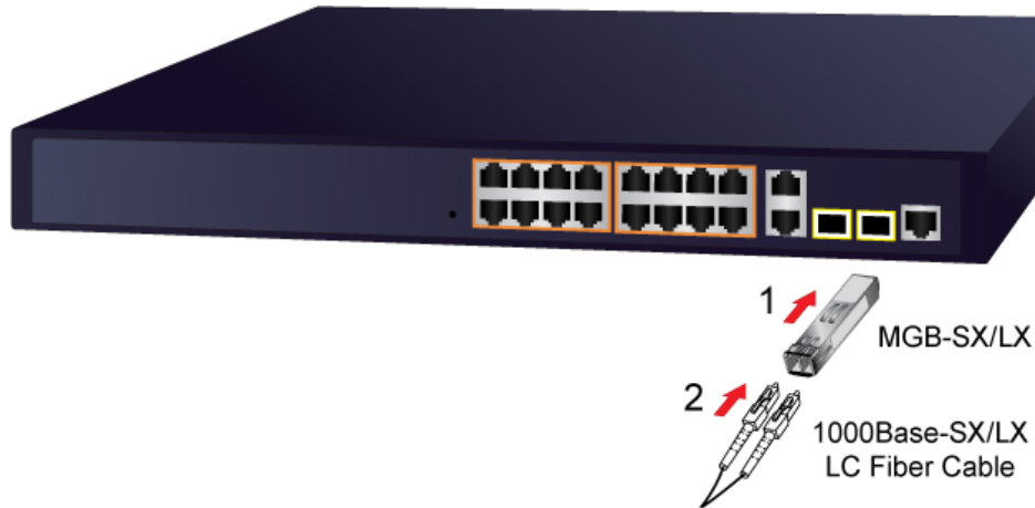
Figure 2-7: Plug-in the SFP Transceiver
