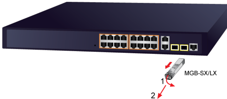
Figure 2-8: How to Pull Out the SFP Transceiver
