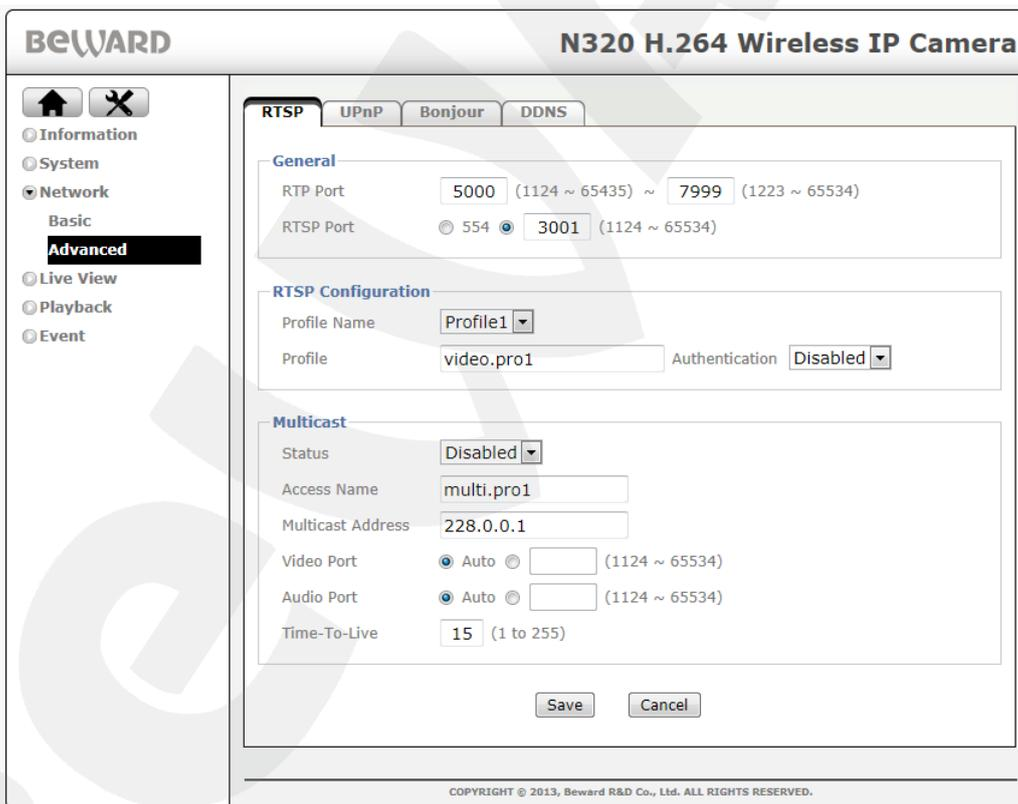
The screenshot shows the configuration page for the BEWARD N320 H.264 Wireless IP Camera. The interface includes a sidebar with navigation options: Information, System, Network (Basic, Advanced), Live View, Playback, and Event. The 'Advanced' option under 'Network' is selected. The main content area is titled 'RTSP' and contains the following settings:
