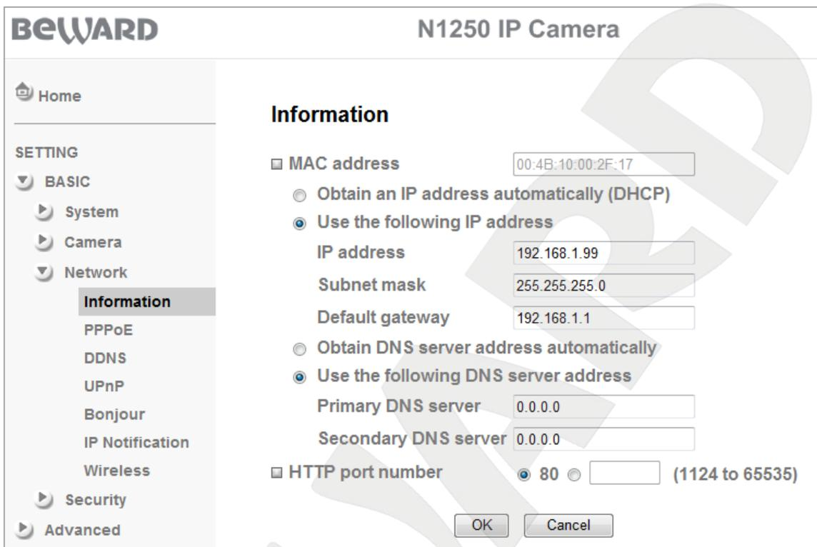
The screenshot shows the BEWARD N1250 IP Camera web interface. The left sidebar contains a 'SETTING' menu with options: Home, BASIC (expanded), System, Camera, Network (expanded), Information (selected), PPPoE, DDNS, UPnP, Bonjour, IP Notification, Wireless, Security, and Advanced. The main content area is titled 'Information' and displays the following settings:
